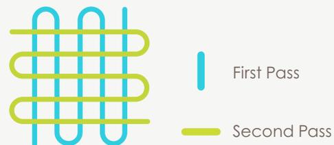
Spray using continuous and parallel strokes overlapping 20% at a constant speed so that an even layer is formed over a section of a large mold or over the whole mold of a smaller size.
